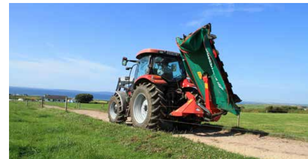
Vertical transport position up to 125°.
