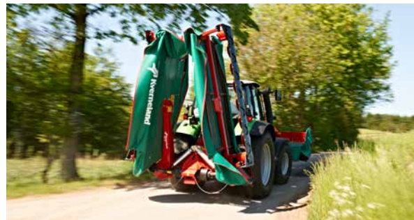
Vertical transport position for good weight distribution.
