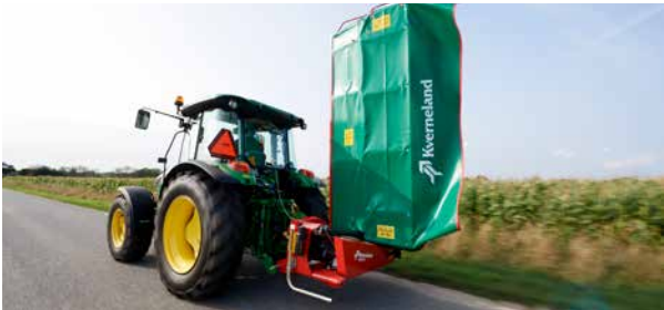
For transport the mower is positioned hydraulically into a vertical transport position.
