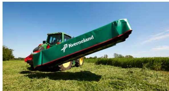
Lifting on headlands via hydraulic cylinder – ample ground clearance.
