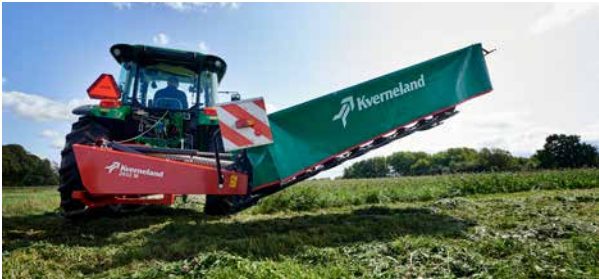
On headlands the mower is lifted without activating the 3pt linkage.
