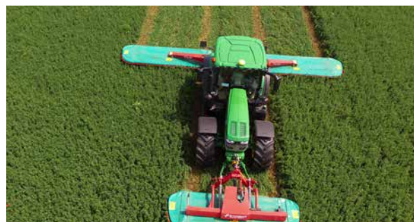
Centre suspended design for excellent ground following ability.
