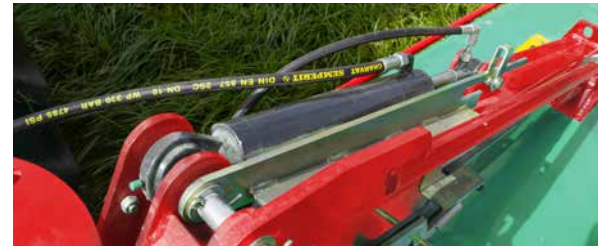
Headland lift via hydraulic cylinder.
